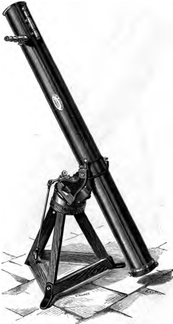
ADJUSTIBLE ALTAZIMUTH OR EQUATORIAL MOUNTING FOR A MEDIUM-SIZED REFLECTOR.
